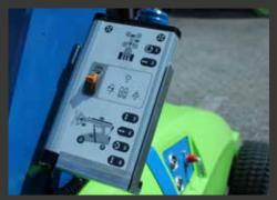
Multifunction control panel in operatorfriendly design with integrated buttons and signal lights, Double action safety keys and Gyro funtionality are both in the standard setup on the Winlet 575.
